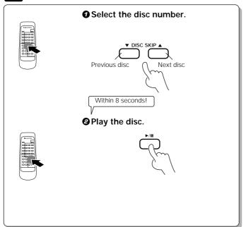
The disc number can be selected directly by using the DISC SELECTOR and numeric keys in place of the DISC SKIP keys.
